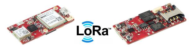
The TM-202 / R9C7 is a high-end product line member of KCS' advanced TraceME track and trace modules. The TM-202 is targeted for remotely tracking and tracing a variety of objects, even livestock, and for personal use.
